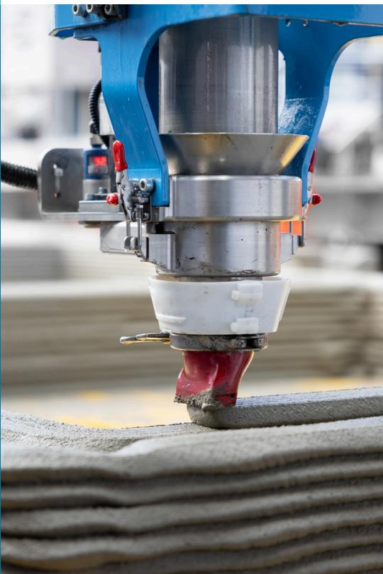
Engineered for next-generation sustainable construction, this biochar-enhanced cementitious composite transforms coconut waste into a carbon-sequestering material optimized for 3D-printed housing and architectural structures.
